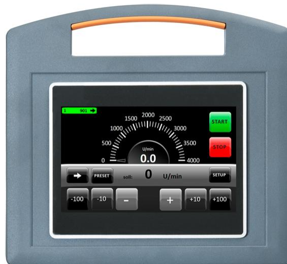
Fig. 3/6: XP20R front with 7" touch display
